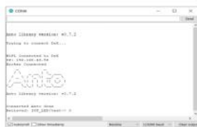
Fig. 7 Esp8266 connected with Anto IoT Platform
